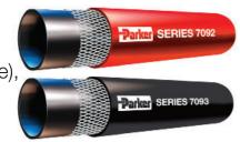
GST® II hose is a versatile general purpose hose designed to handle air, mild chemicals and water. The hose construction incorporates a tube that is compatible with light oil mists found in air tool lubricating systems, and the multiple plies of textile reinforcement provide flexibility. The cover is resistant to abrasion, heat and ozone, and is available in multiple standard colors for color-coded identification.
